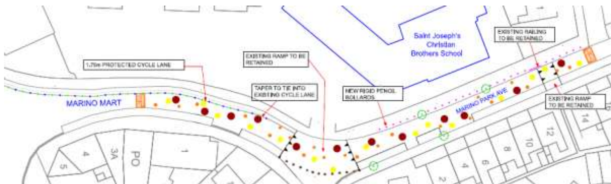
Image 3: Extent of the works at St. Joseph's CBS Primary School Marino Mart and Marino Park Avenue
