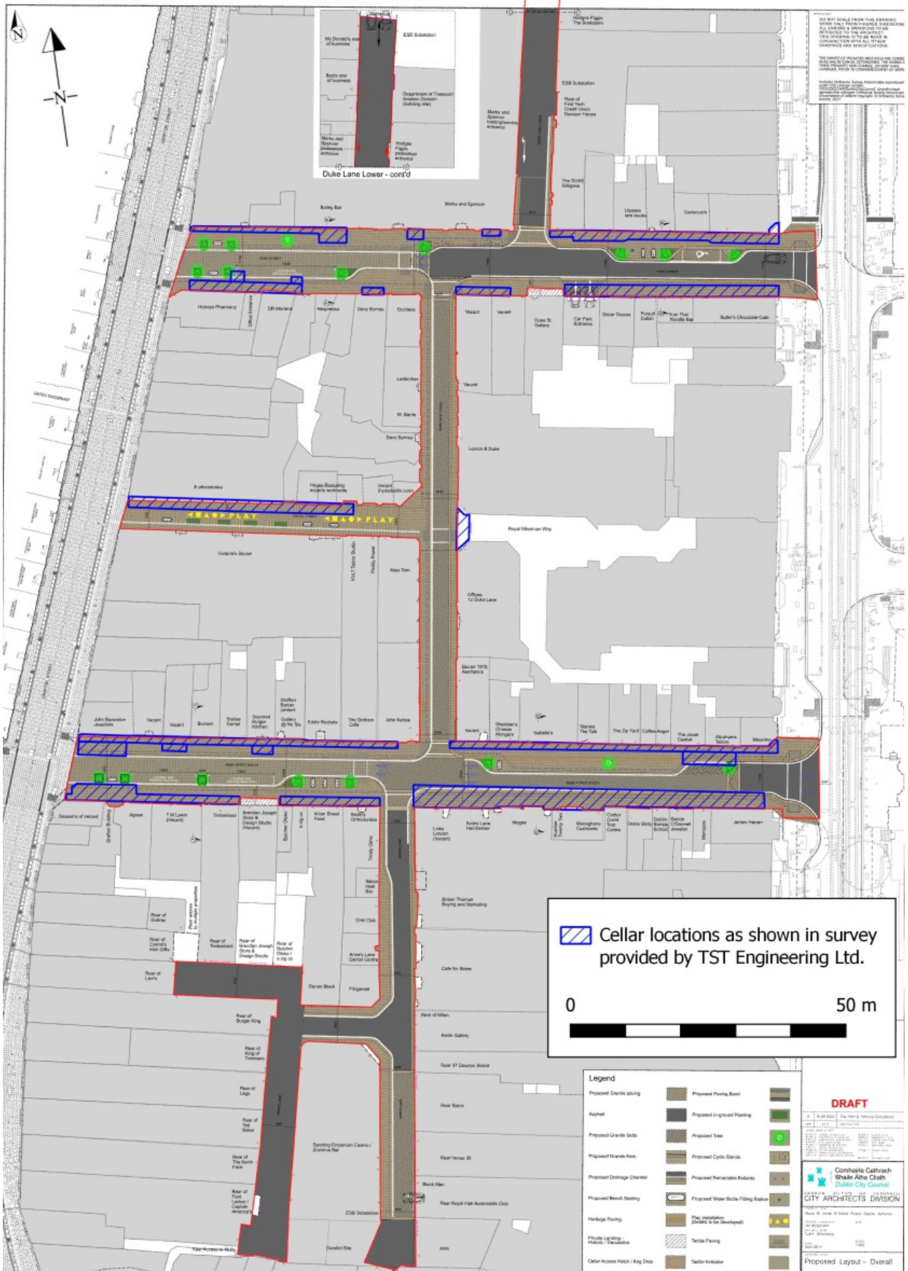
Location of basement/cellars from TST Engineering LTD GPR Survey (2015)
