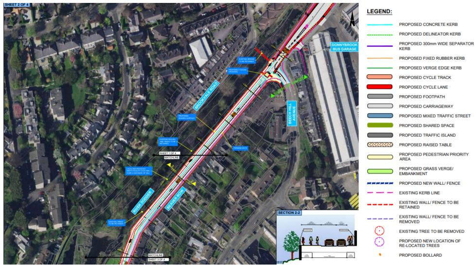
Figure 3 Donnybrook Rd to Clonskeagh Rd Rapid Deployment Scheme 2/4 Source: Cycling Design Office. A full scaled version of the drawing is available separately.
