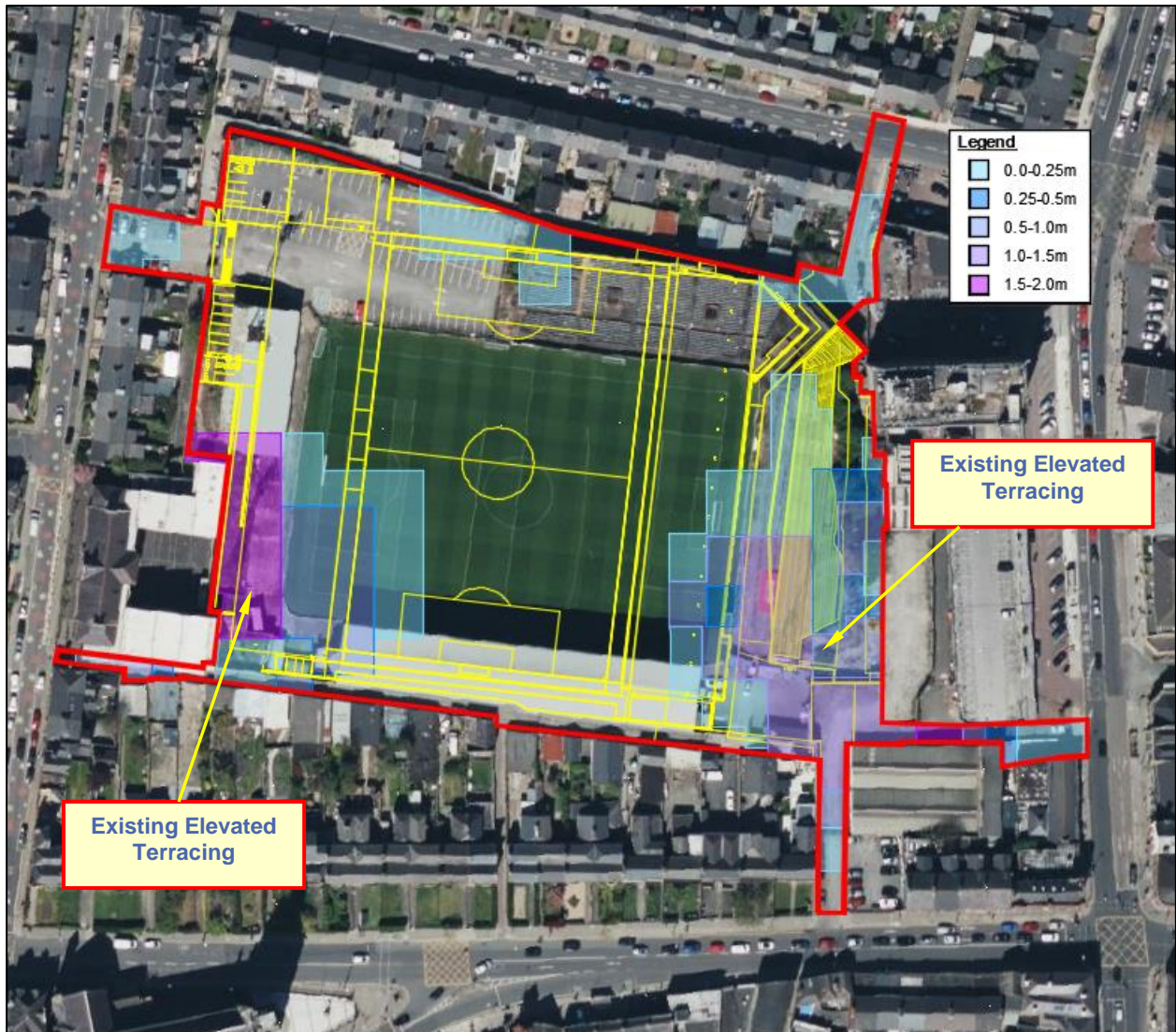
Figure 15 – Dublin Pluvial Study – 0.5% AEP (1 in 200 year) Pluvial Flood Extent Depth Mapping Overlaid onto Proposed Site Layout
