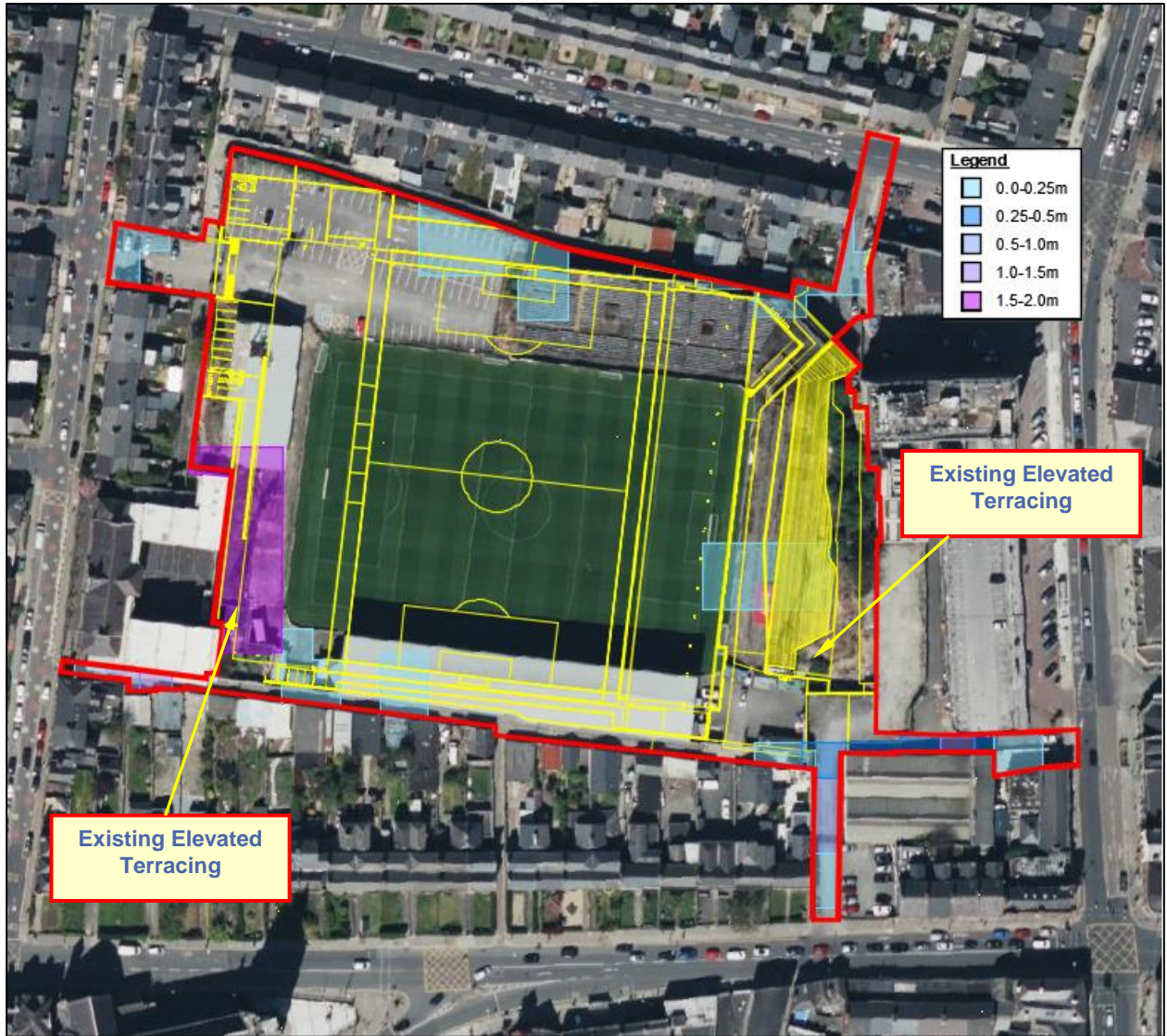
Figure 13 – Dublin Pluvial Study - 10% AEP (1 in 10 year) Pluvial Flood Extent Depth Mapping Overlaid onto Proposed Site Layout
