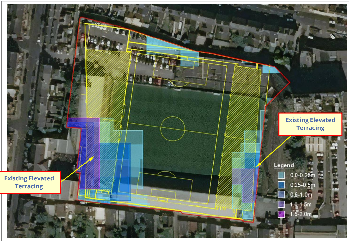
Figure 15 – Dublin Pluvial Study – 0.5% AEP (1 in 200 year) Pluvial Flood Extent Depth Mapping Overlaid onto Proposed Site Layout
