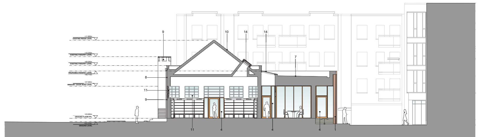
PROPOSED SECTION SHOWING THE NEW ROFFLIGHT INTO THE EXISTING LIBRARY PITCHED ROOF
