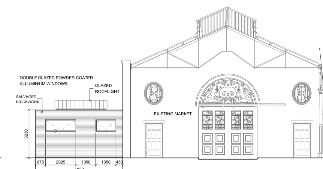
Proposed Side Elevation of New Toilet Block
