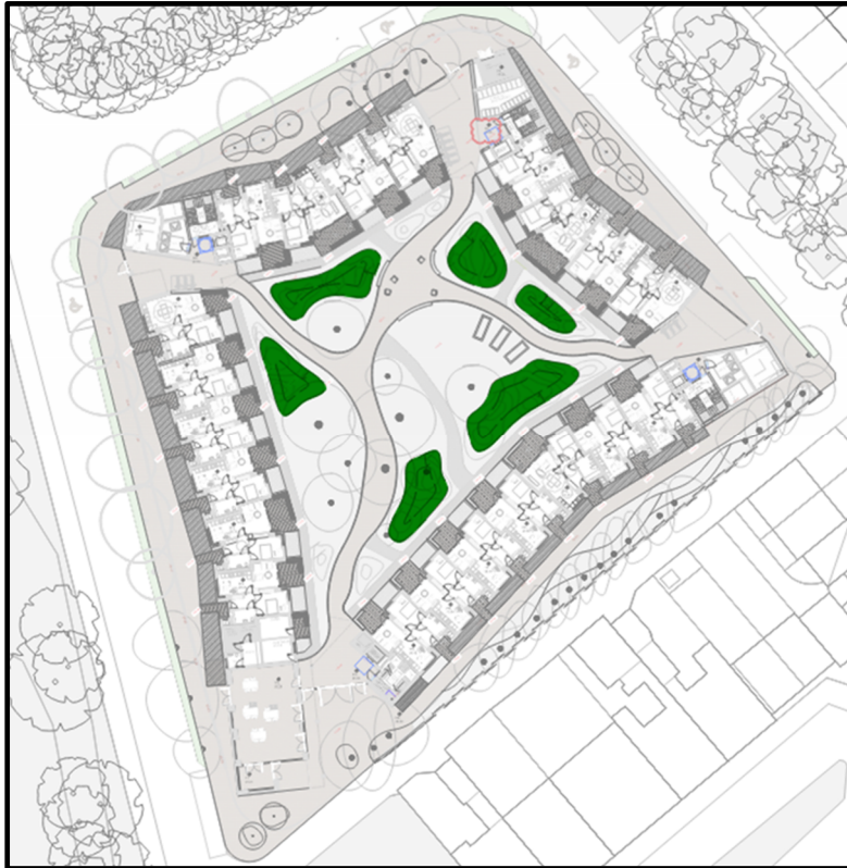
Figure 11: Planted swales and extent of this SuDS feature on site
