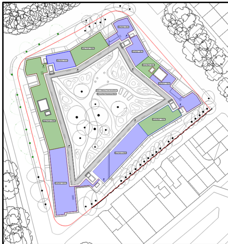
Figure 12: Green and blue roofs and extent of these SuDS feature on site
