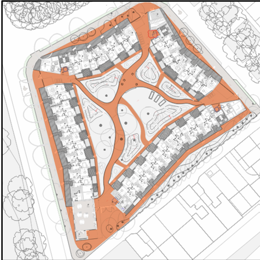
Figure 13: Permeable paving and extent of this SuDS feature on site
