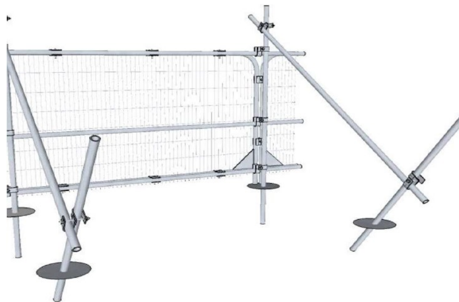
Figure 1: Tree Protection Fencing
