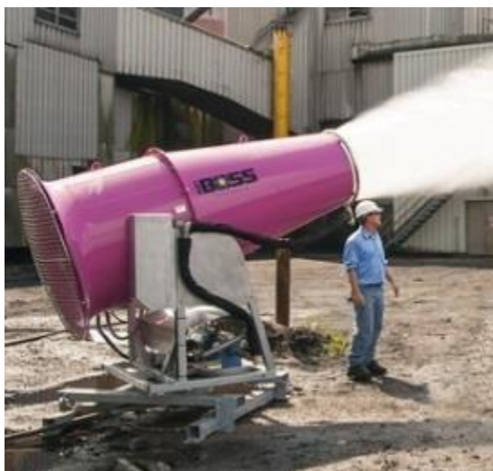
Figure 3-2: Dust Suppression System
