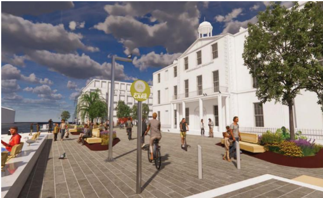
The proposed layout separates pedestrians from cyclists at the junction with Richmond Street South through the use of street furniture
