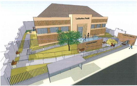
Fig 21 – Proposed new arrangement with entrance platform, landscaped accessible ramp, also symmetrical stepped access.
