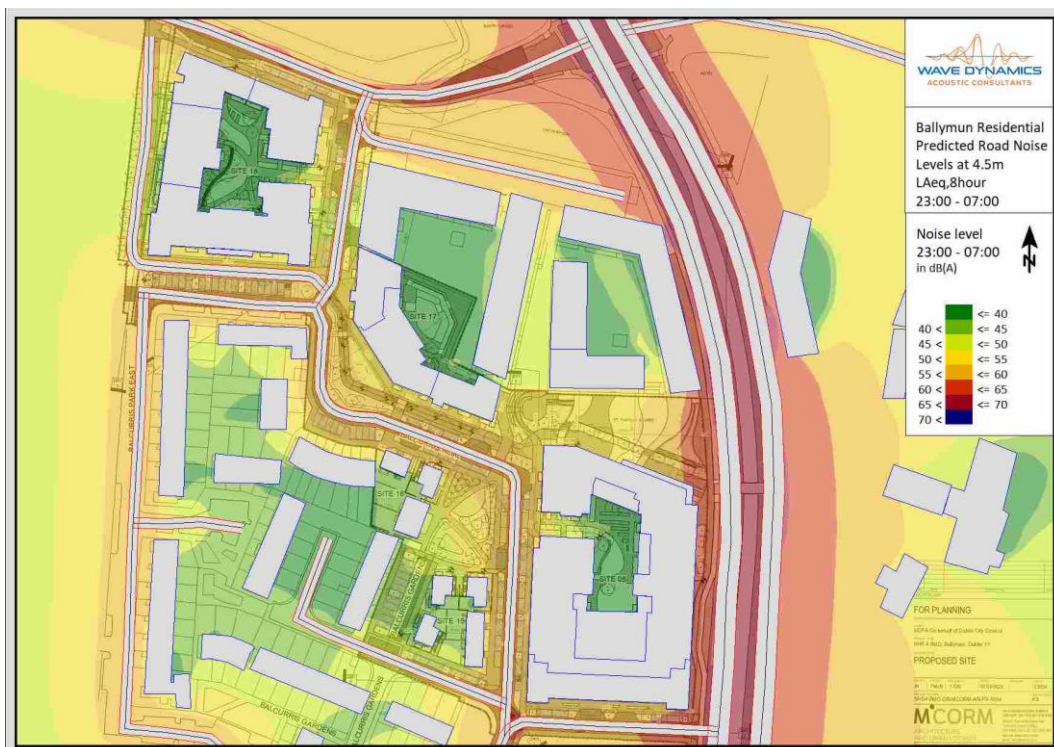
Figure 11: Predicted road noise L_{Aeq,8hour} (23:00Hrs – 07:00Hrs) at 4.5m height for the future development.
