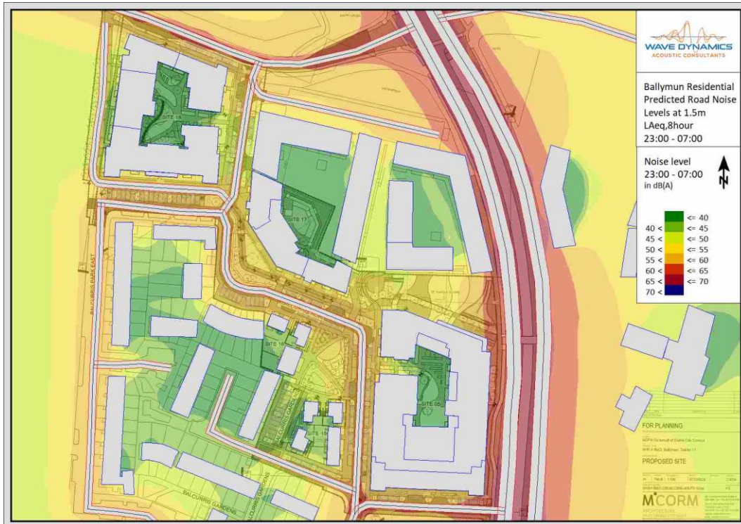
Figure 10: Predicted road noise L_{Aeq,8hour} (23:00Hrs – 07:00Hrs) at 1.5m height for the future development.
