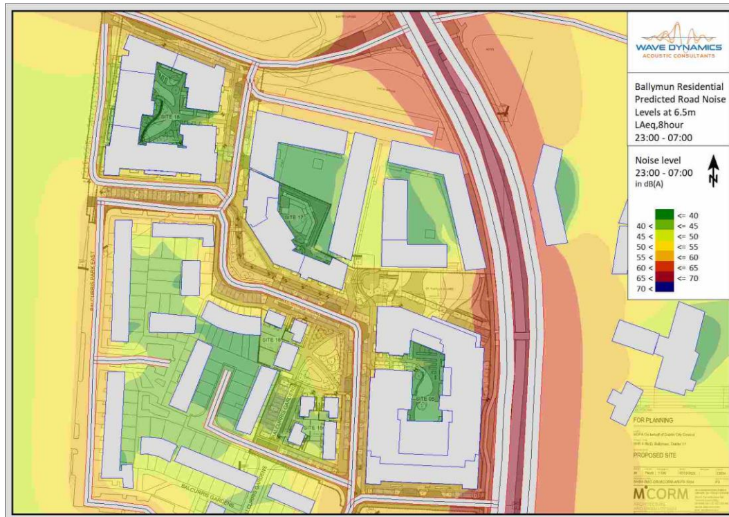
Figure 12: Predicted road noise L_{Aeq,8hour} (23:00Hrs – 07:00Hrs) at 6.5m height for the future development.
