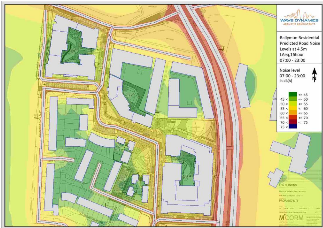
Figure 8: Predicted road noise L_{Aeq,16hour} (07:00Hrs – 23:00Hrs) at 4.5m height for the future development.
