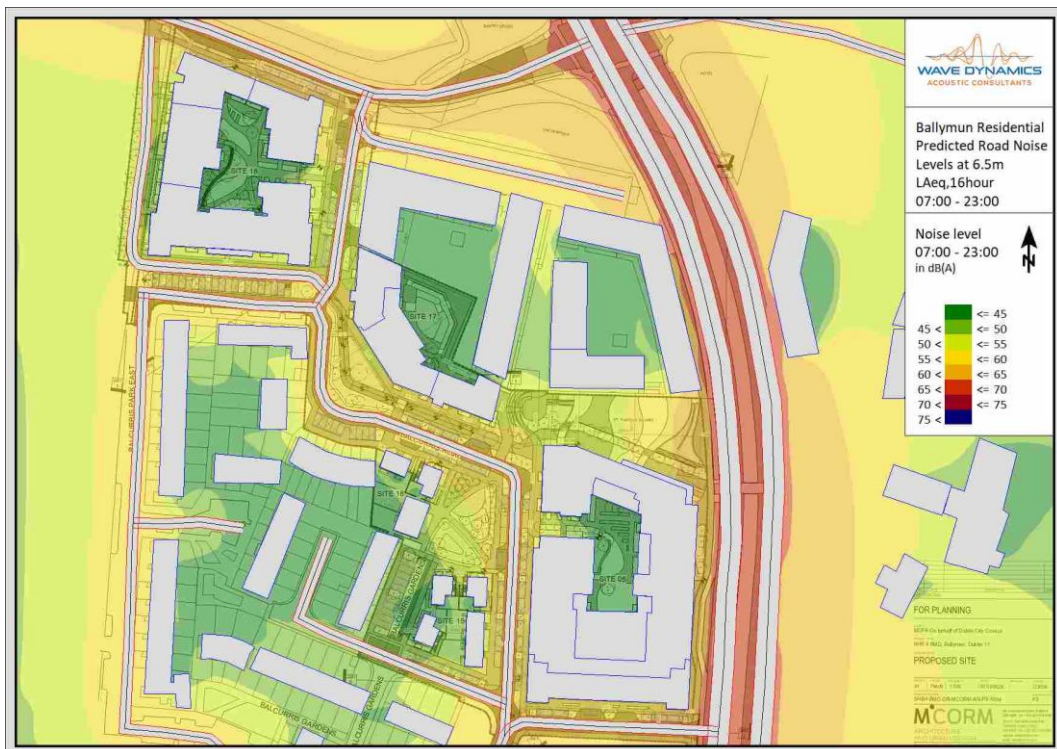
Figure 9: Predicted road noise L_{Aeq,16hour} (07:00Hrs – 23:00Hrs) at 6.5m height for the future development.
