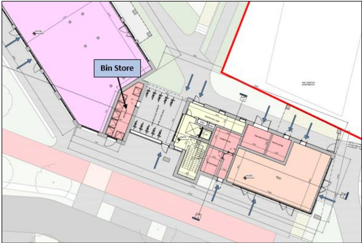
Figure 3.0 Waste Storage Areas – Site 17
