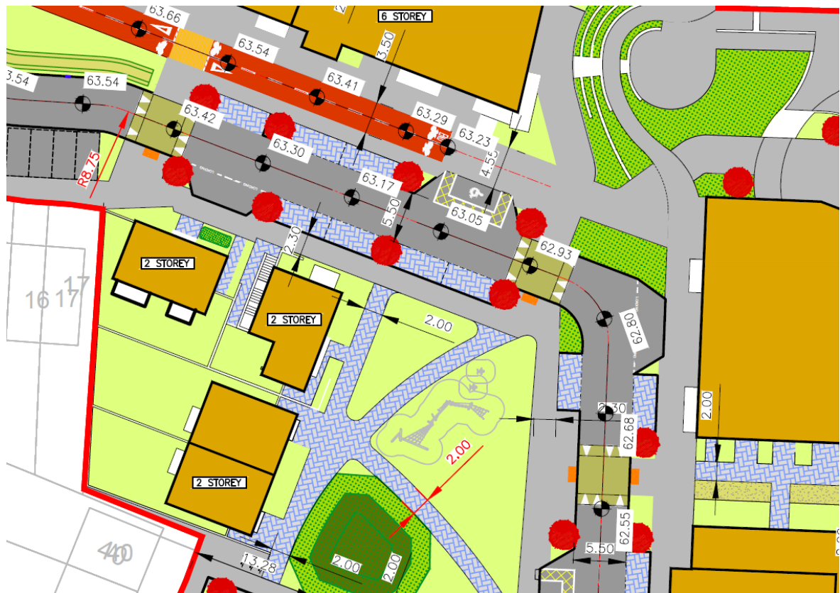
Figure 6.1 – Proposed Trees and parking compromising intervisibility of pedestrians and motorist at crossings
