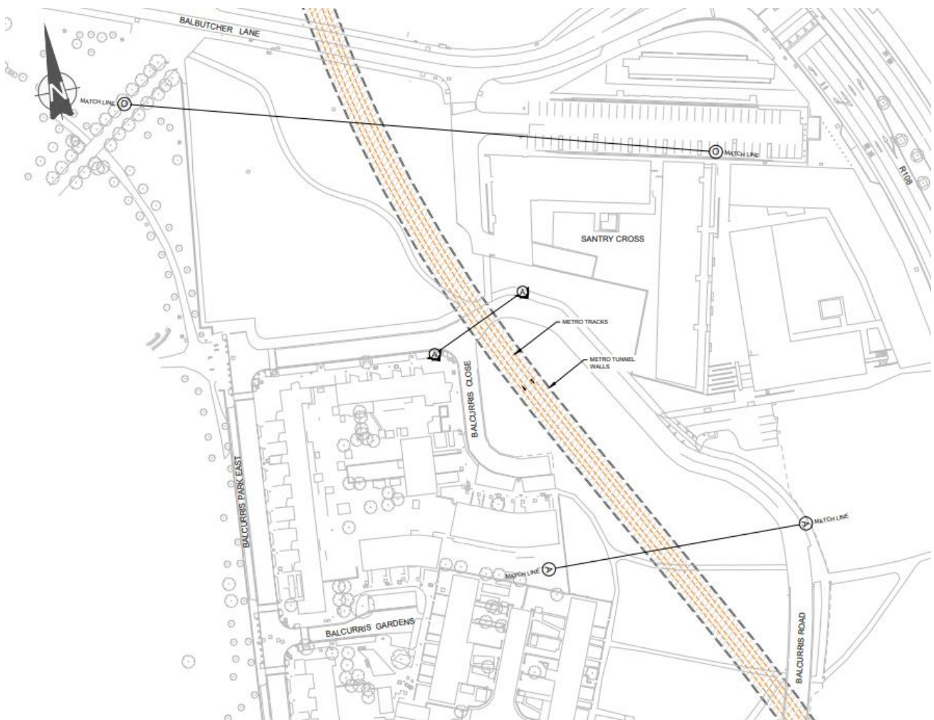
Figure 14: General Arrangement showing alignment of the MetroLink tunnel below the site (Source Jacobs & IDOMS as displayed on An Bord Pleanála's website)
