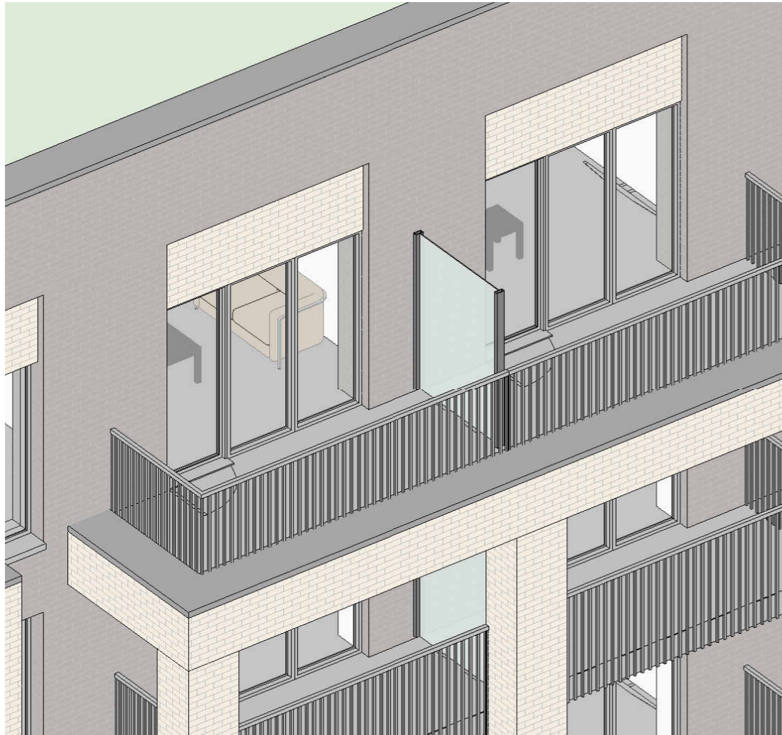
Image 81 - Typical Balcony Detail illustrating privacy screens
