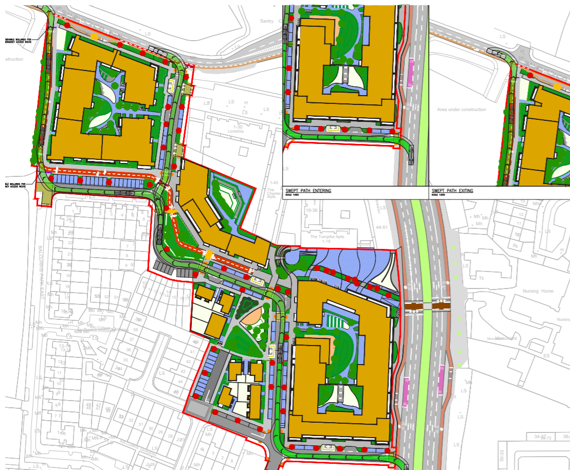
Image 107 - Swept Path Analysis- Aerial Platform Special Appliance
