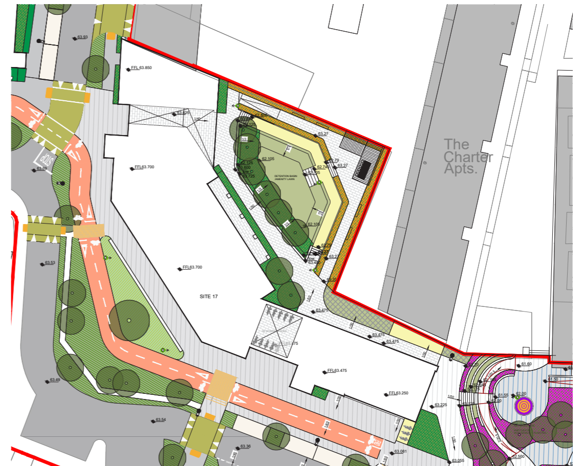
Image 60: - Site 17 Site Plan defining new areas of quality public realm on Balcurris Road and St. Pappin's Square as well as a private courtyard- Ground finishes flow under the access archways to the cores and courtyard
