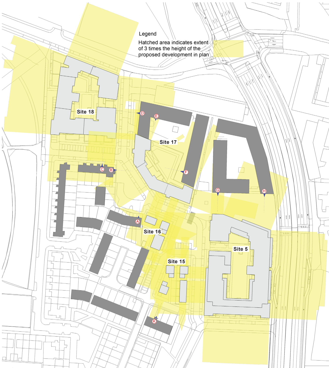
Figure 2: Proposed site plan showing the zone of influence (3 times the height of the proposed building) and direction of the window wall of adjacent residential properties.
