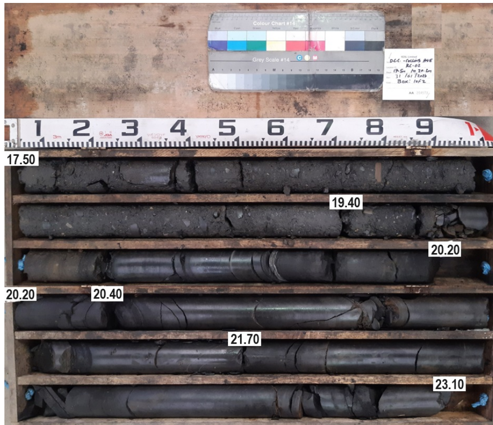
Figure 7 – Bedrock cores in RC02 from 17.50-23.10m with transition from CLAY (Glacial Till) to ROCK at 19.40m bgl (28.61m OD).
