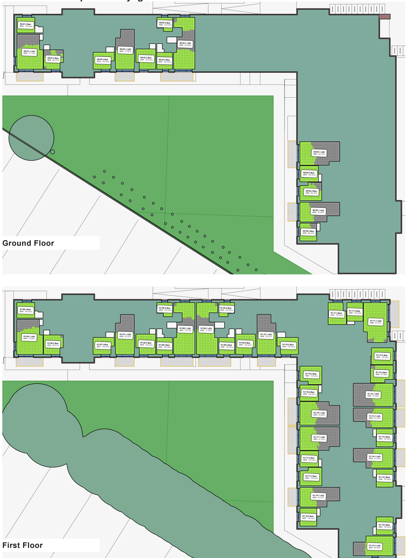
Figure 31: Block A - Floor plans indicating Daylight Provision to BS EN17037:2021+A1 Table NA.1
