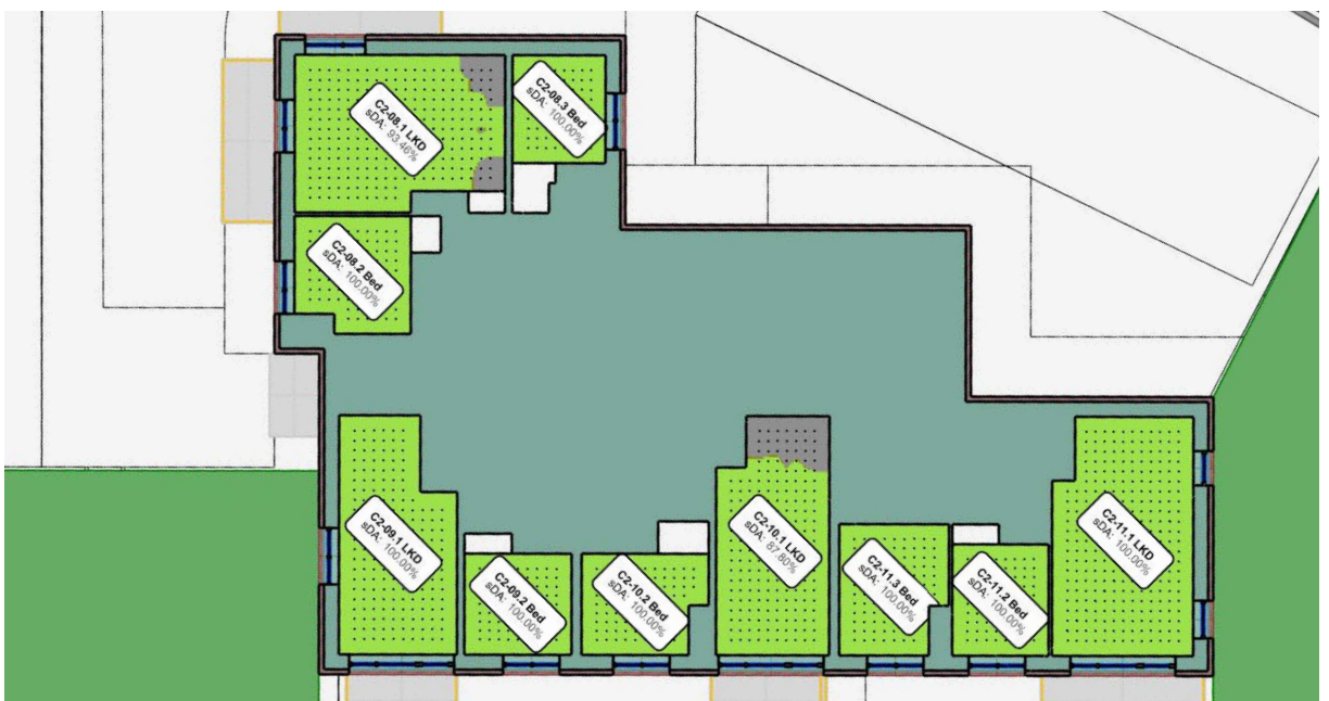
Figure 29: Block C - Floor plans indicating Daylight Provision to BS EN17037:2021+A1 Table NA.1
