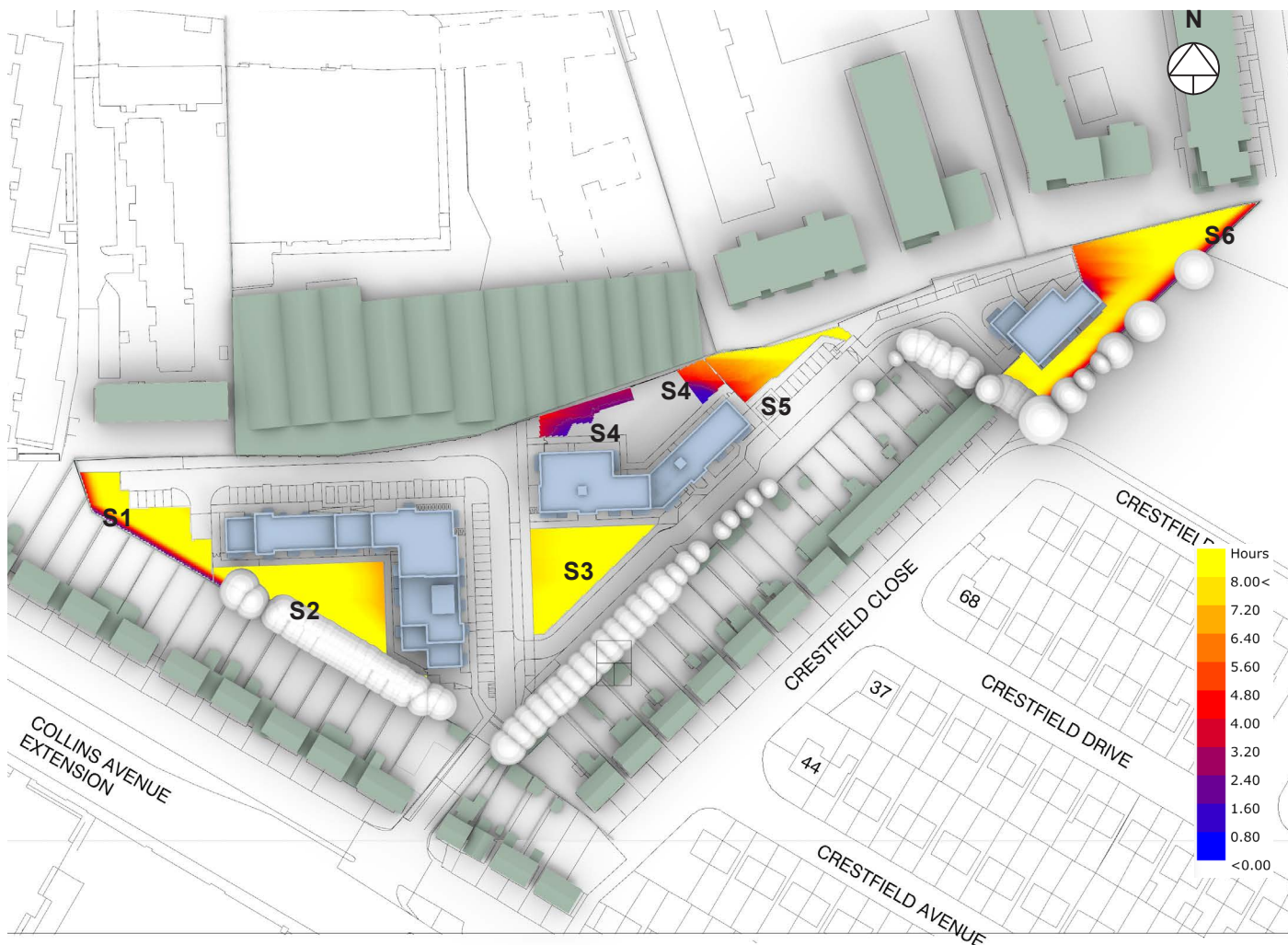
Figure 8: Communal Open Space - Radiation map of amenity area, showing available sunlight on 21st March. The scale represents the percentage of daylight received from 0 - 8 hrs.
