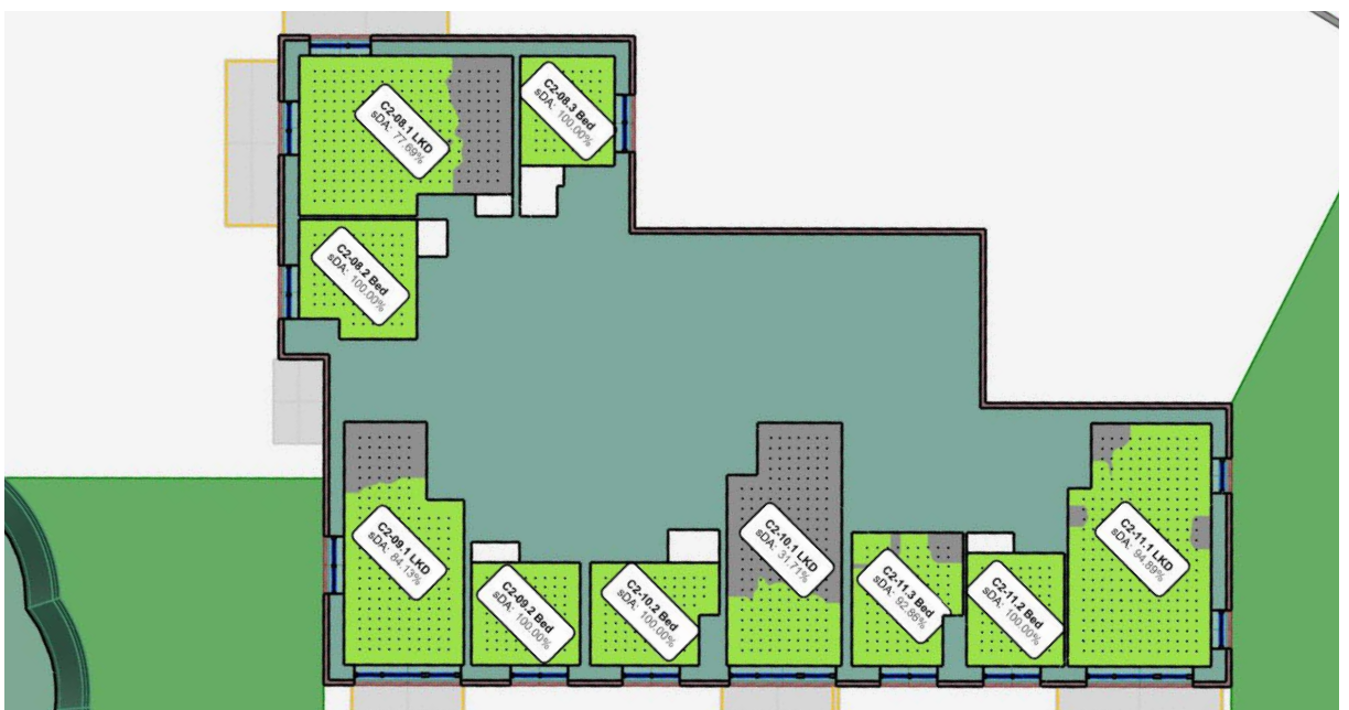
Figure 36: Block C - Floor plans indicating Daylight Provision to BS EN17037:2021+A1 Table NA.1
