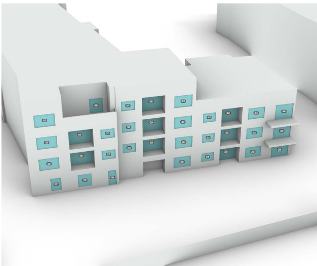
Figure 5: Milner’s Square Block E: View of model locating VSC and APSH test points.
