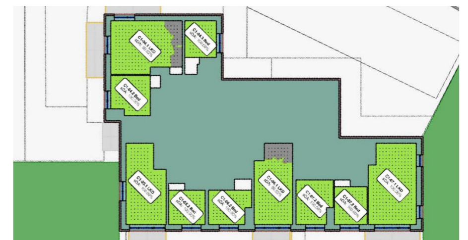
Figure 64: block C minimum room specific daylight provision
