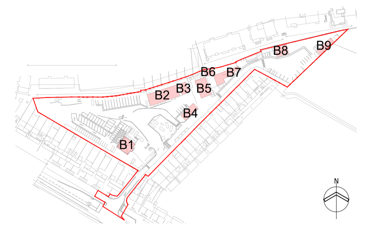
Existing Buildings to be demolished
