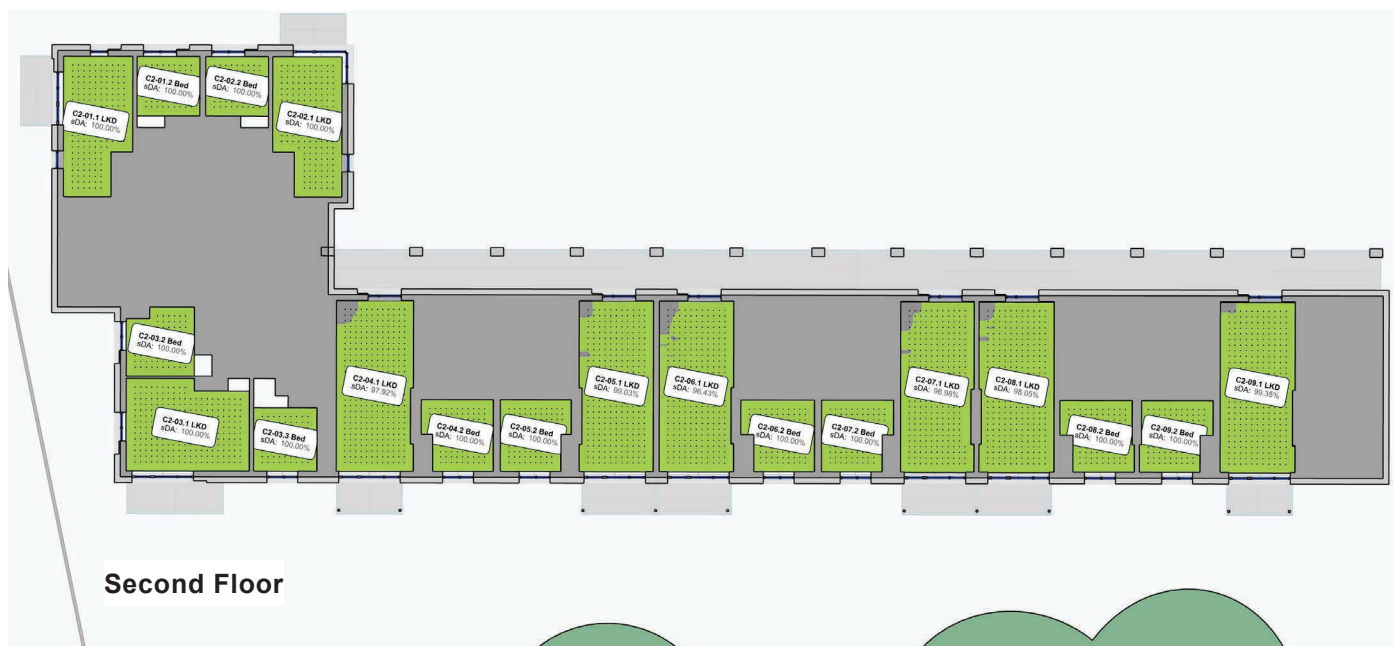
Figure 36: Block C - Floor plans indicating Daylight Provision to BS EN17037:2021+A1 Table NA.1 Assessment with existing trees in place
