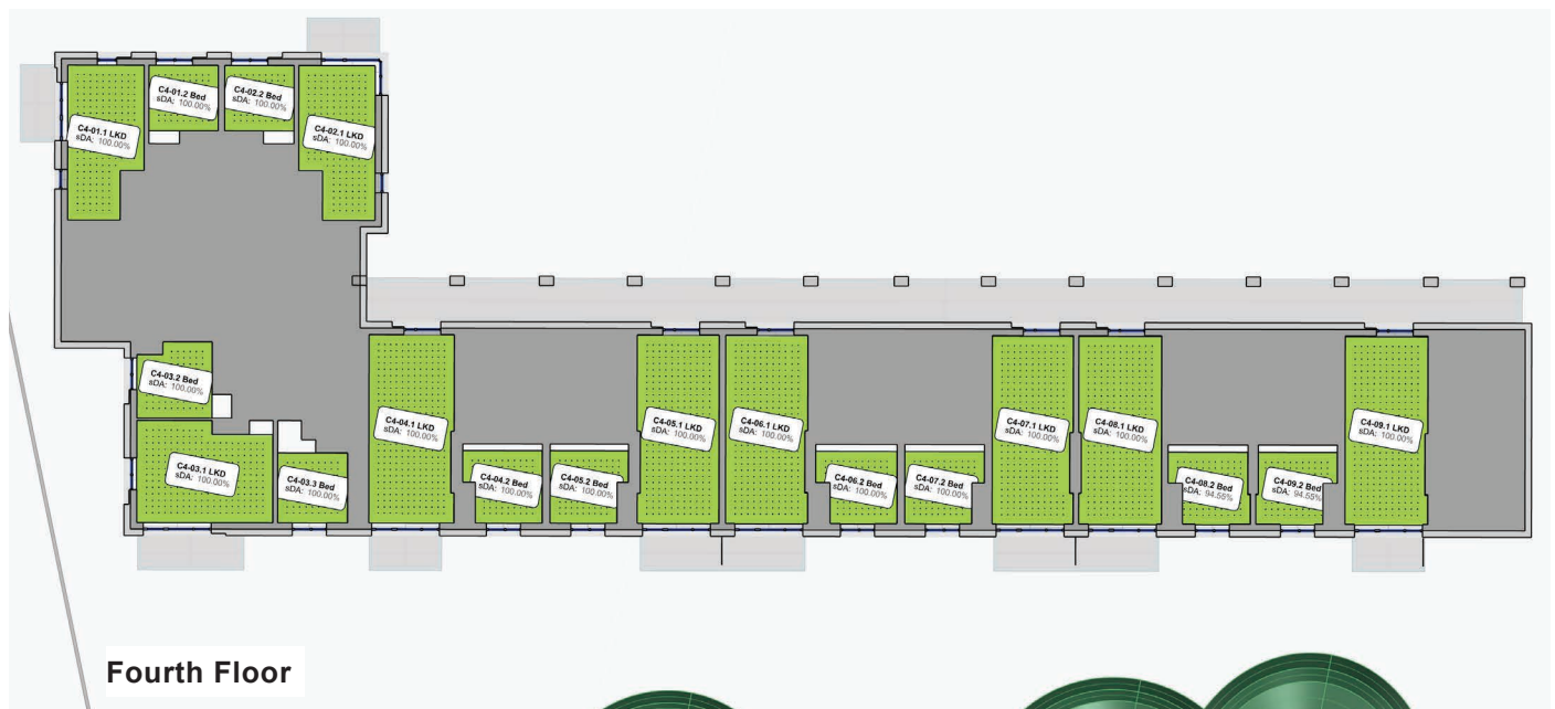
Figure 37: Block C - Floor plans indicating Daylight Provision to BS EN17037:2021+A1 Table NA.1 Assessment with existing trees in place
