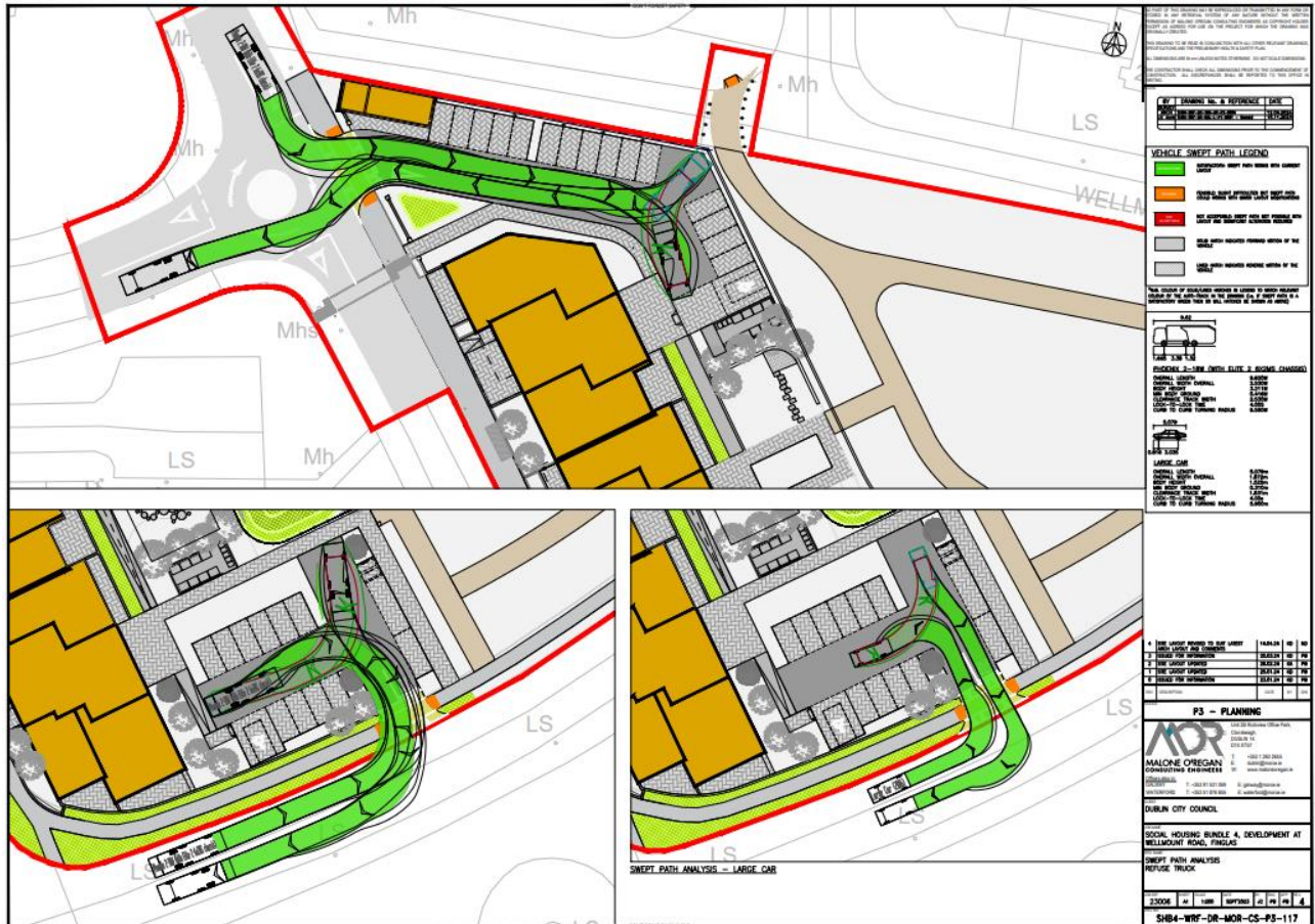
Figure 2.0 Swept Path Analysis Refuse Truck
