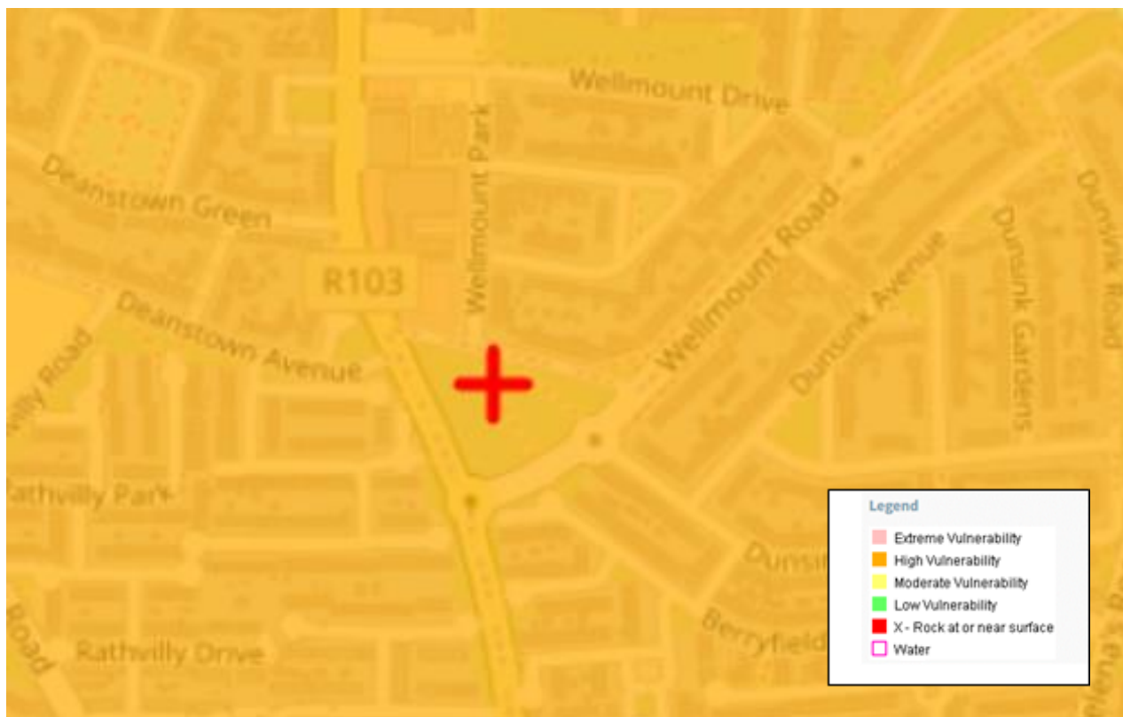
Figure 7: Ground Water Vulnerability (Source: EPA Maps)
