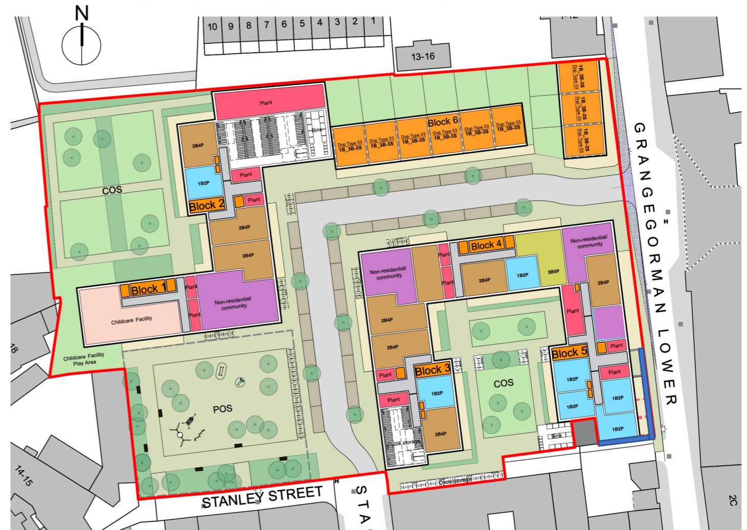
Above: Ground Floor Plan – retention of existing structures to south-eastern corner of site, shown in dark blue
