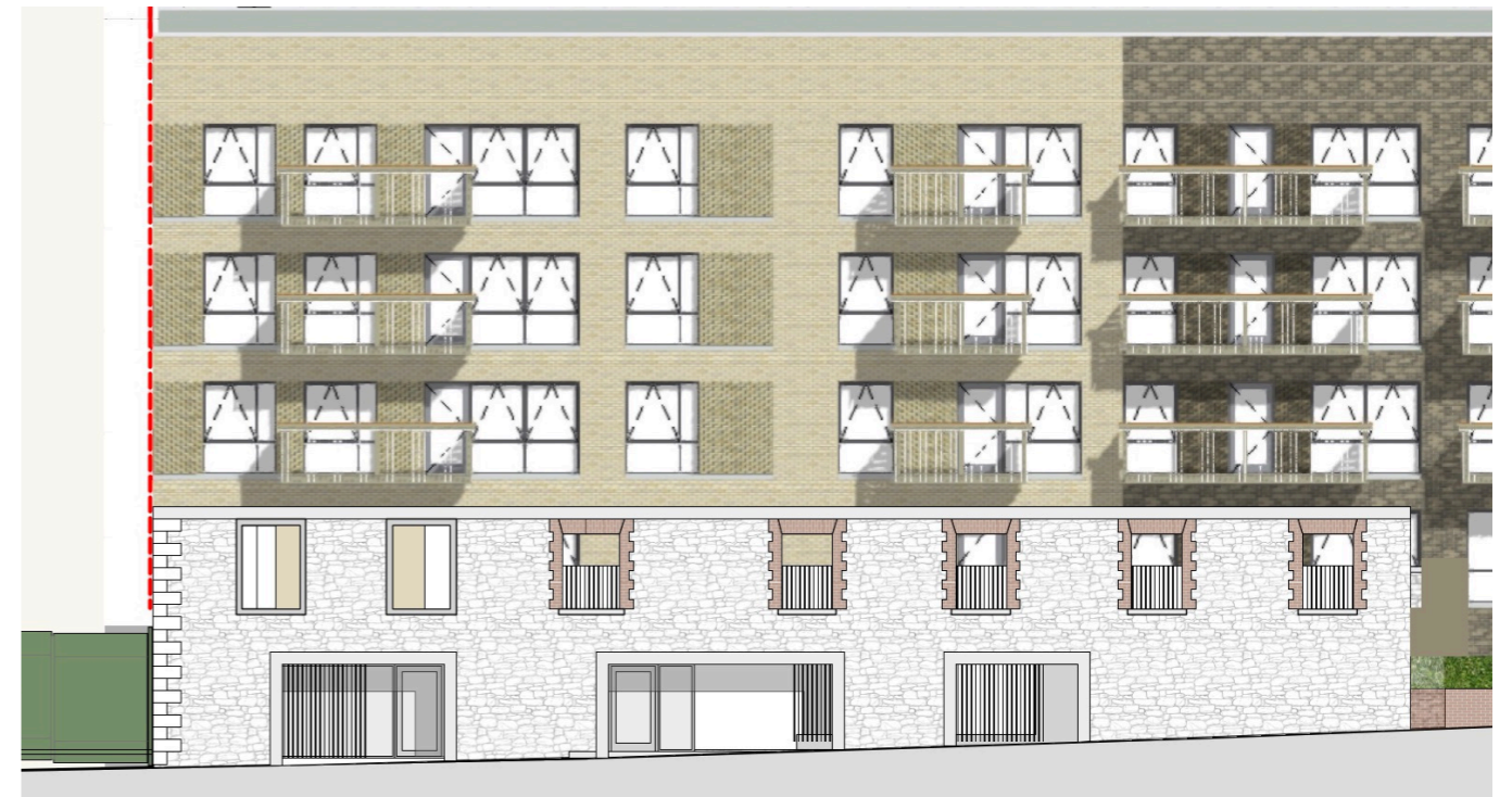
Above: Developed elevation study, showing retention of existing openings and the formation of new contemporary openings, in particular at street level.
