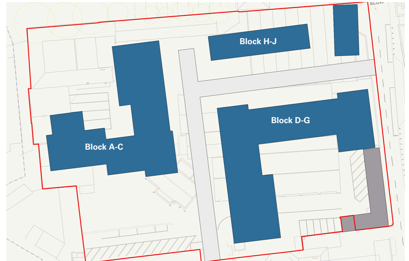
Above: Study option, showing the retention of Building 03 (in grey) with development of the remainder of the site as per Site Strategy Option 02&03. This proposal proved unviable for a number of reasons, in particular as it would result in the loss of c.20no. apartments, and would challenge the project's viability.
