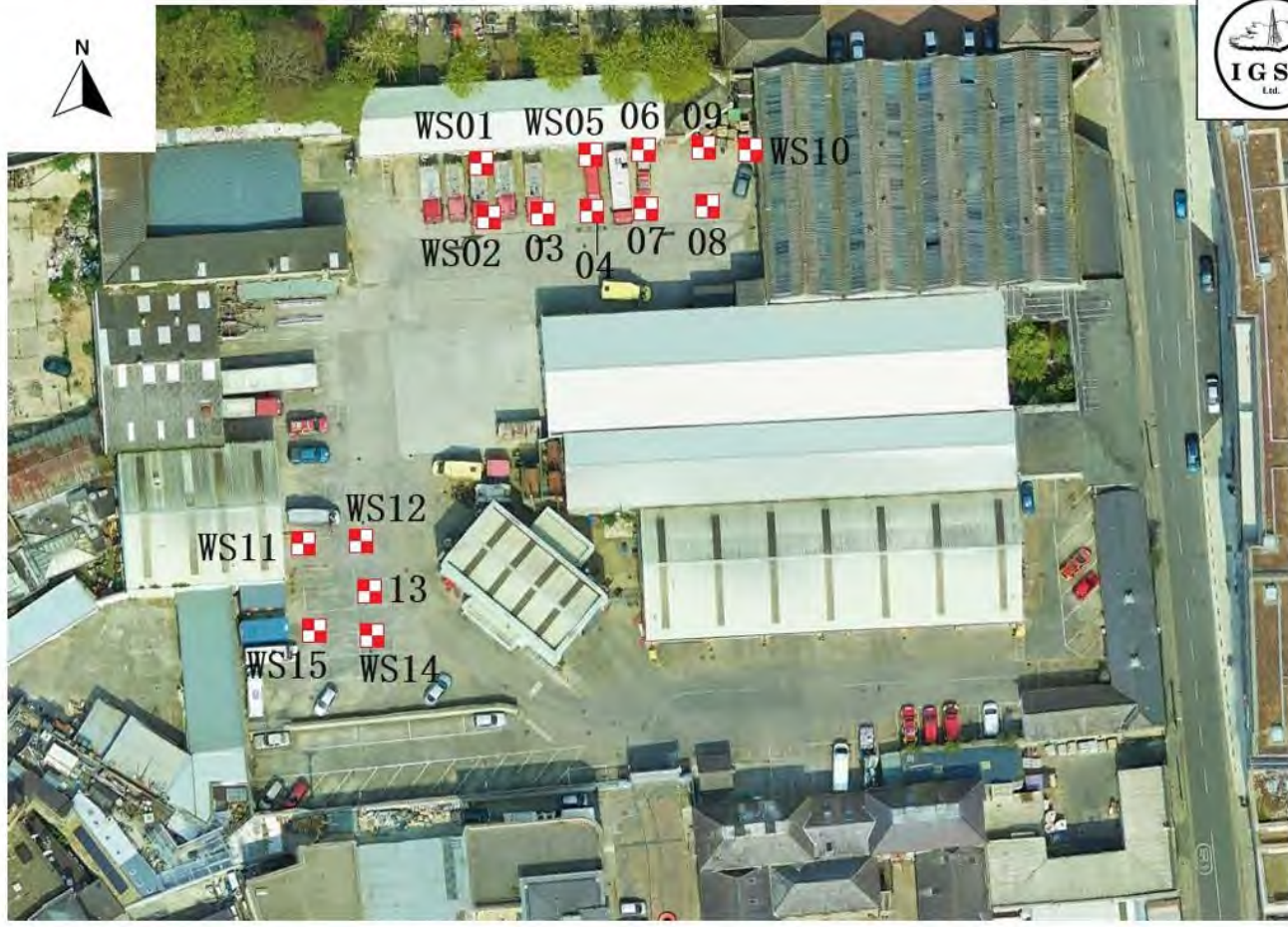
25000-1 - Exploratory Hole Site Plan – Window Samples (WS01-WS15)
