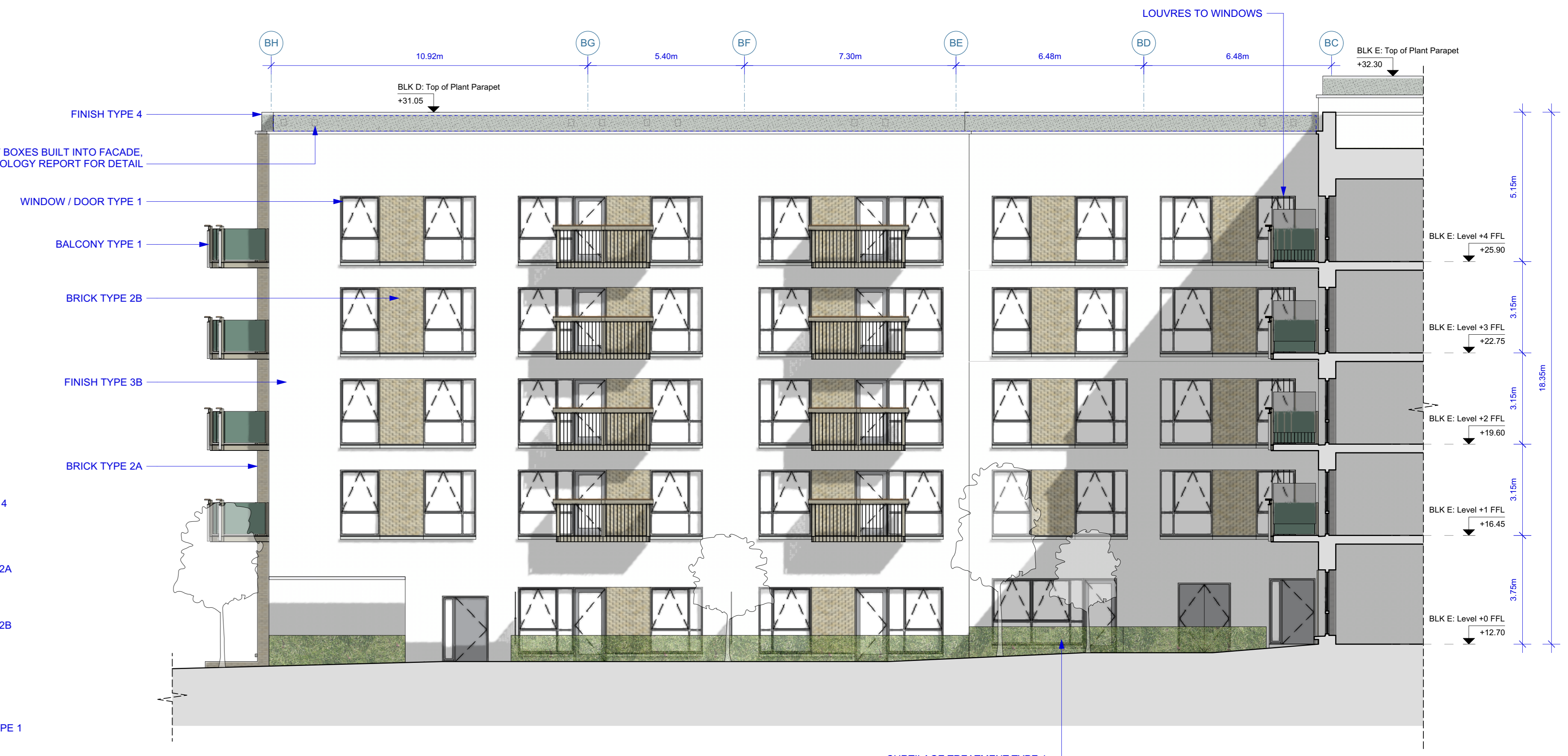
3 Building 2 Internal Courtyard Elevation - East Elevation Scale: 1:100
