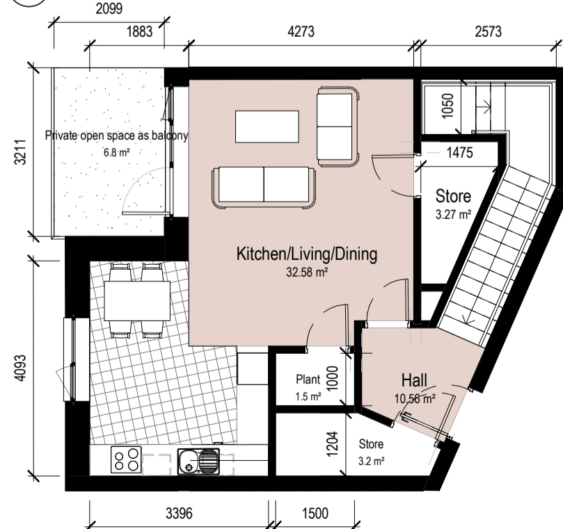
3 2 Bedroom Duplex Unit Type D1 Ground Floor Plan 1 : 100
