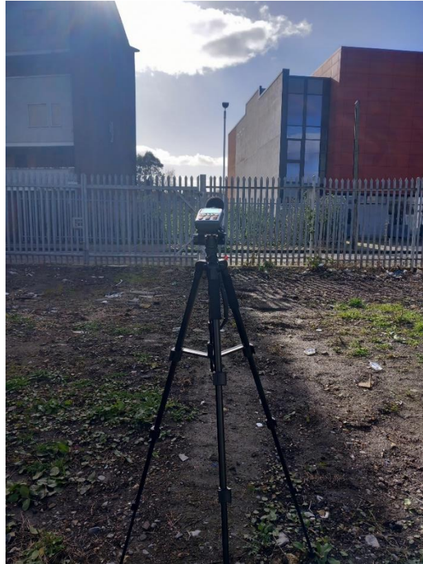
Figure 5: Attended Measurement Setup.
