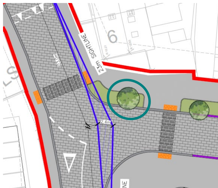
Figure 5.6 – Stopping Sight Distance compromised by tree
