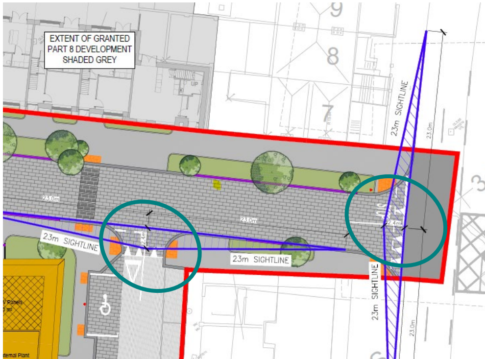
Figure 5.1 – Raised Crossings without drainage detail
