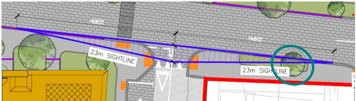
Figure 5.5 – Visibility Splay interrupted by tree
