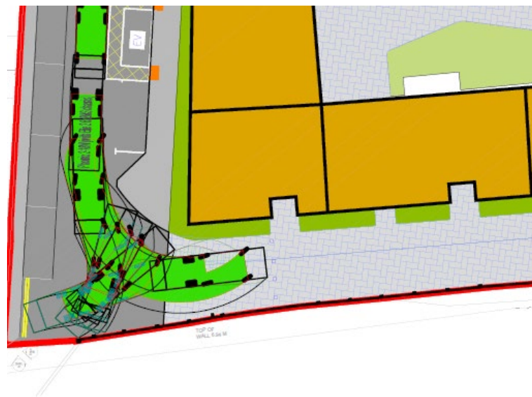
Figure 5.9 – Large vehicle making a turnabout manoeuvre
