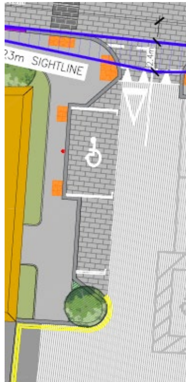
Figure 5.3 – Parking bays without drainage detail
