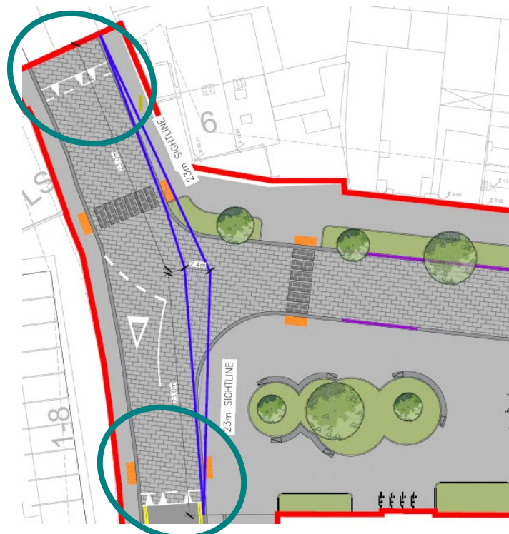
Figure 5.2 – Raised Crossings without drainage detail
