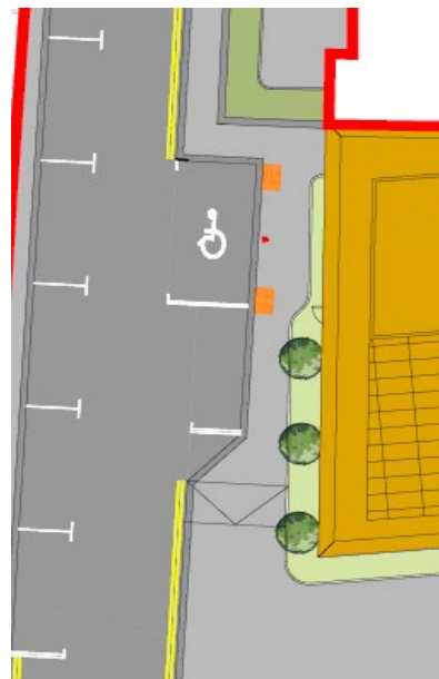
Figure 5.4 – Parking bays without drainage detail
