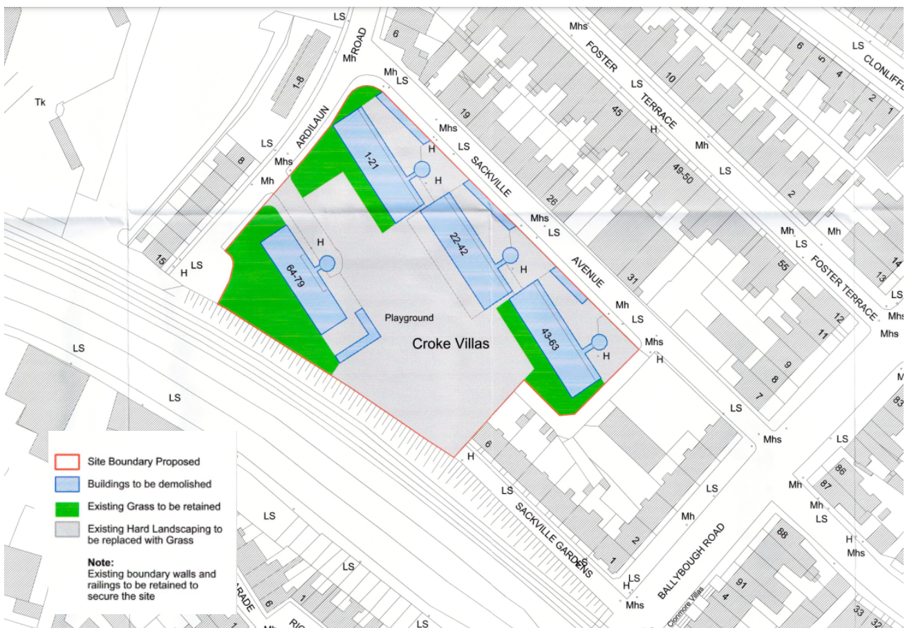
Figure 7: Proposed Demolition Plan (Source: DCC)
