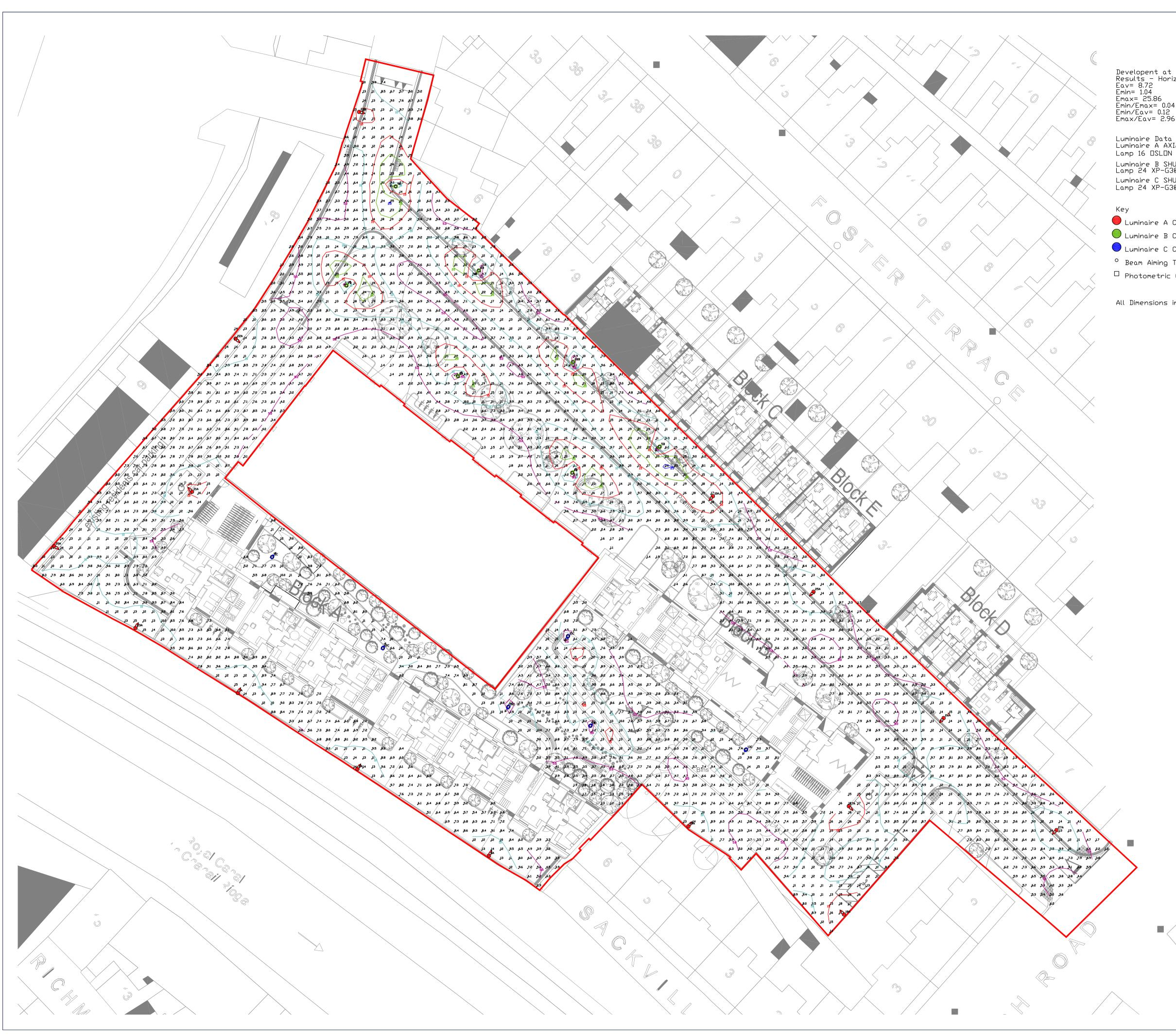
Developent at Croke Villa's Result's - Horizontal Illuminance (lux) Eav= 8.72 Emin= 1.04 Emax= 25.86 Emin/Emax= 0.04 Emin/Eav= 0.12 Emax/Eav= 2.96
