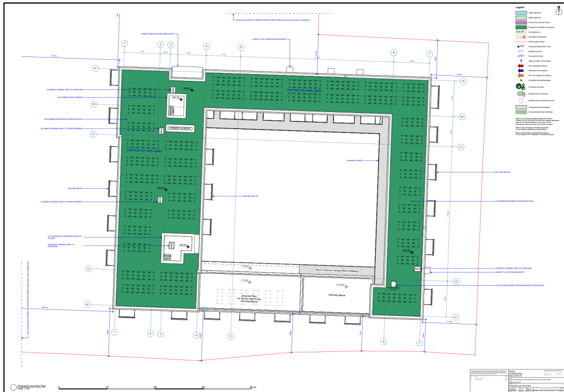
Figure 2: Extract from drawing “SHB4-CAF-DR-SHA-AR-P3-1005-Proposed Level Roof Plan” showing the proposed roof layouts with the location of the proposed PV panels.
