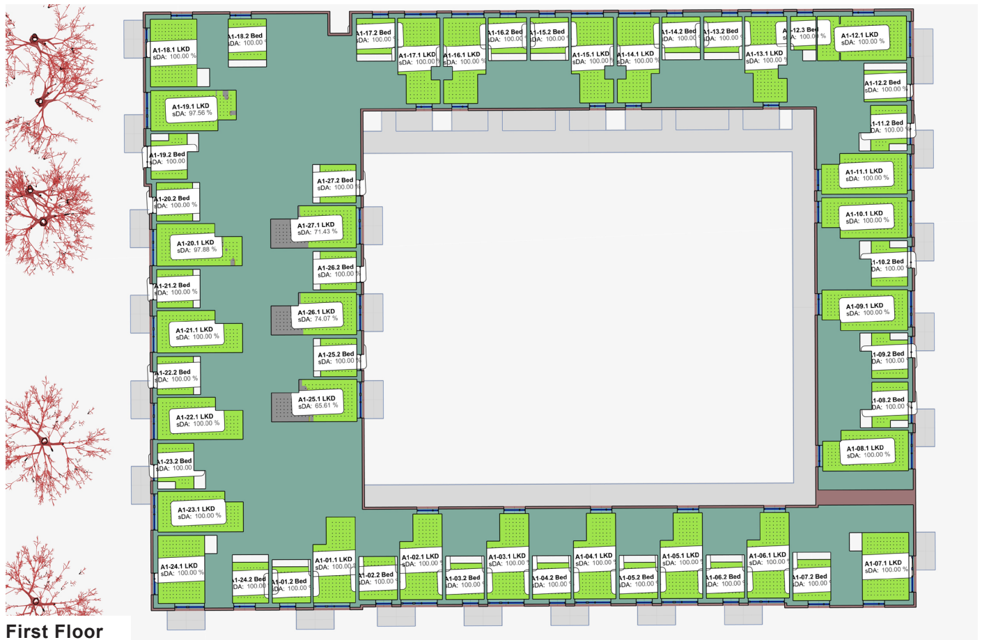
Figure 22: Floor plans indicating Daylight Provision compliance to BS EN17037:2021+A1 Table NA.1. Results shown in the winter condition.
