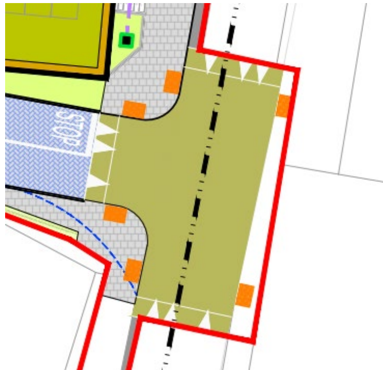
Figure 5.2 – Raised Crossings without drainage detail
