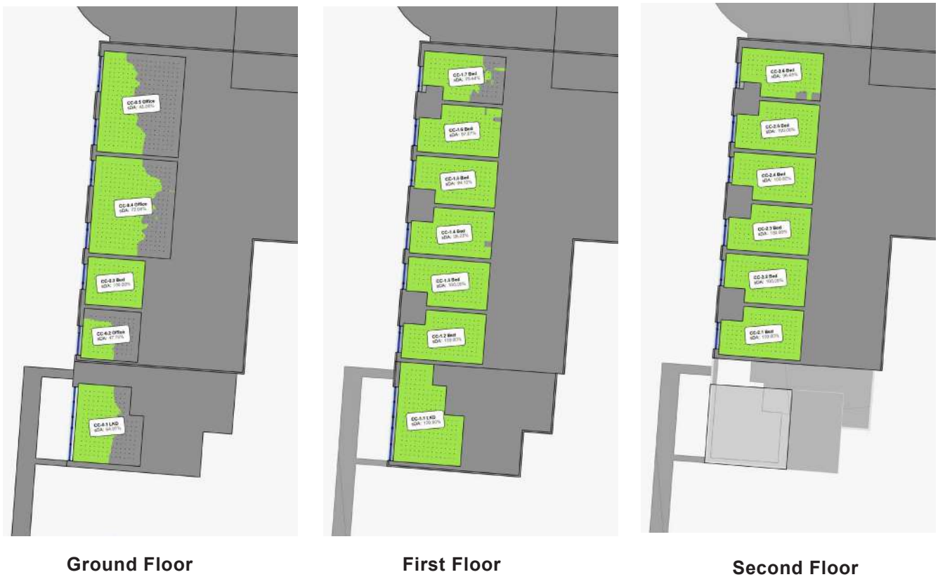
Figure 9: BS EN17037:2018+A1:2021 Minimum room specific Daylight Provision in accordance with UK National Annex Table NA.1.
