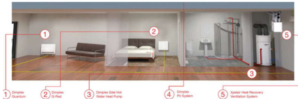
Figure 3: Typical smart electric system.
