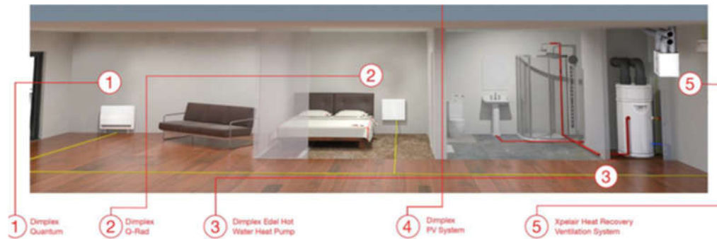
Figure 3: Typical smart electric system.
