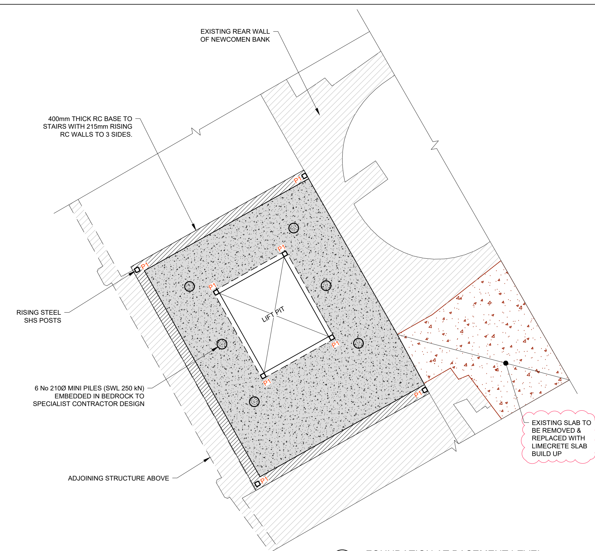
1 FOUNDATION AT BASEMENT LEVEL SCALE 1:50
